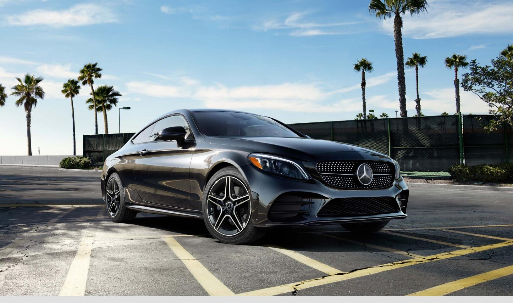
C 300 Coupe SPECIFICATIONS /ENGINE 2.0L inline-4 turbo /POWER 255 hp @ 5,800 rpm /0-60 MPH  $\rightarrow$  5.9 sec<sup>15</sup> /DRIVE rear-wheel or 4MATIC® all-wheel /SUSPENSION selective-damping /WHEELS 18" twin 5-spoke
